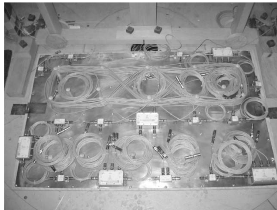
Figure 5. 1553 network on copper ground plate
